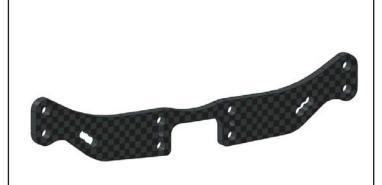
This product is a new setting part that aims to improve the grip feeling by reducing the rigidity between the bulkhead tops of the damper stay and to improve the handling stability in high grip conditions. T4 2019 For rear.
