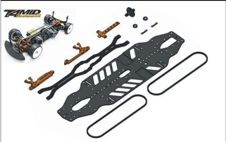
This product is a conversion kit based on XRAY T4 '17  $\sim$  ' 19. The purpose of the development is to reduce the time lag during throttle operation as much as possible by eliminating the belt front-back difference and to facilitate operation.
