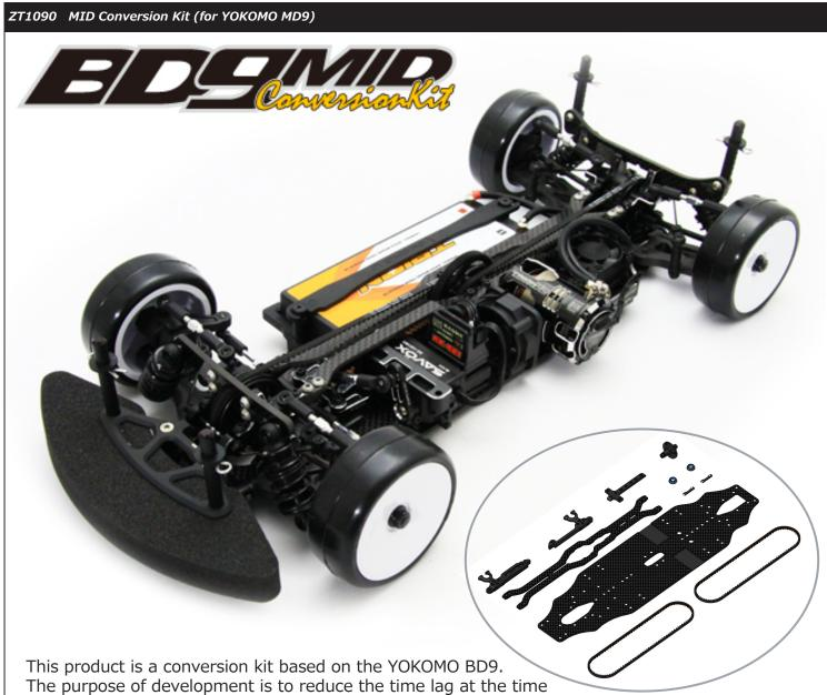
of throttle operation as much as possible by eliminating the difference in belt length between front and back. As a result, the motor is laid out on the center side, enabling a balanced midship layout to be realized.
